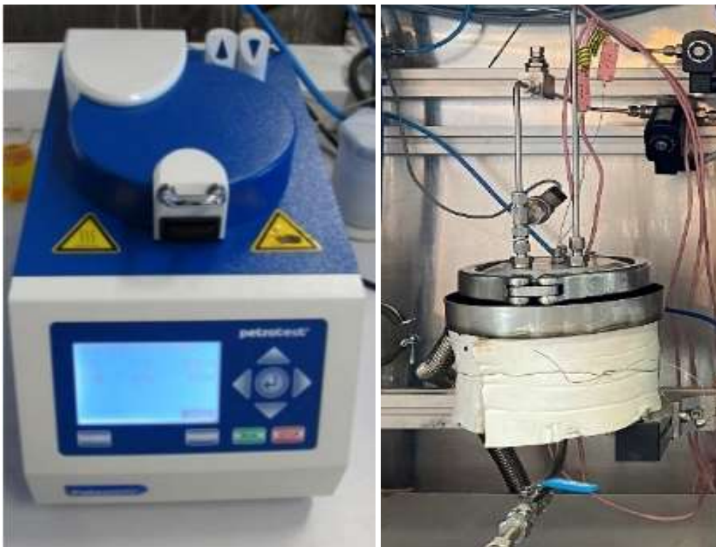
Figure 8: Standard test method "PetroOxy" and reactor in "BigOxy" test rig.
