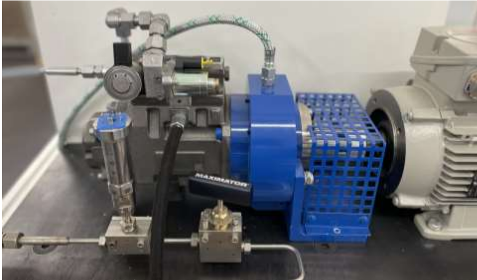
Figure 10: Test bench set-up with high-pressure pump connected to the throttle and a pressure sensor.
