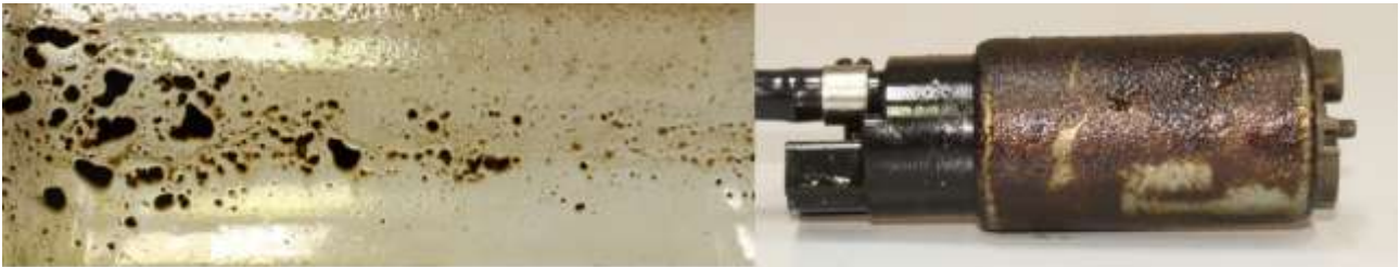
Figure 13: The fuel sediments in the tank and on the low pressure pump from test run with 10 % Bio-HFO.
