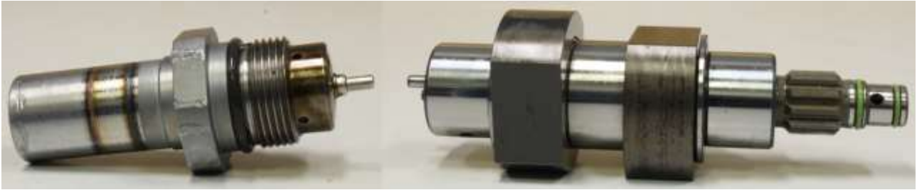
Figure 12: The High pressure pump components from test run with 10 % Bio-HFO.
