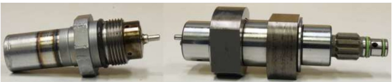
Figure 4: The High pressure pump components from test run with 10 % Bio-HFO.
