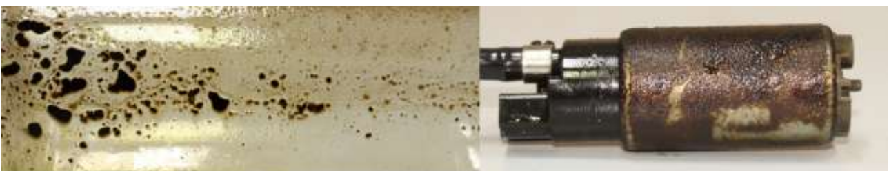
Figure 5: The fuel sediments in the tank and on the low pressure pump from test run with 10 % Bio-HFO.
