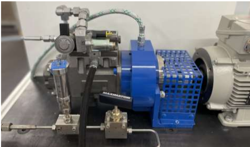
Figure 2: Test bench set-up with high-pressure pump connected to the throttle and a pressure sensor.
