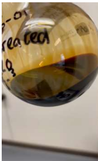
Figure 6. Final Bio-HFO product produced from BTG-3042 hydrotreated CLO sample at BTG continuous flow reactor.
