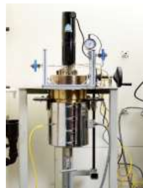
Figure 7. Bench scale 4 L Hastelloy reactor for Bio-HFO production.
