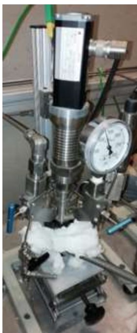
Figure 1. (left) Reactor setup used by CSIC to develop lab-scale recipe. Reaction conditions: Volume 25mL; Feed volume 14 mL; Lignin amount in CLO 9 wt%; 5wt% Ru/C catalyst amount 0.441 g (40% with respect to lignin); Temperature 250 °C; initial pressure 30 bar H 2 ; reaction time 22h. (right) Molecular weight analysis of CLO before and after the HDO process depicting also the maximum operating pressure in the reactor.
