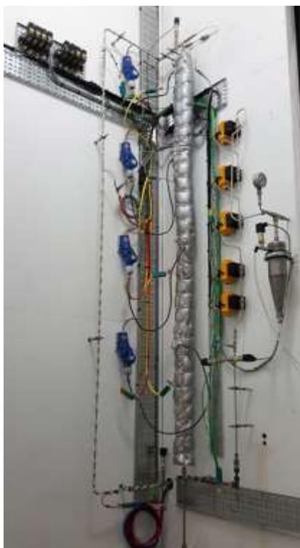
Figure 4. (left) bench scale hydrotreaters that were used for Phase A of BTG contract; (right) Battery limits for material handling with Vertoro handling the hydrotreated CLO for methanol evaporation and analysis of final Bio-HFO product.
