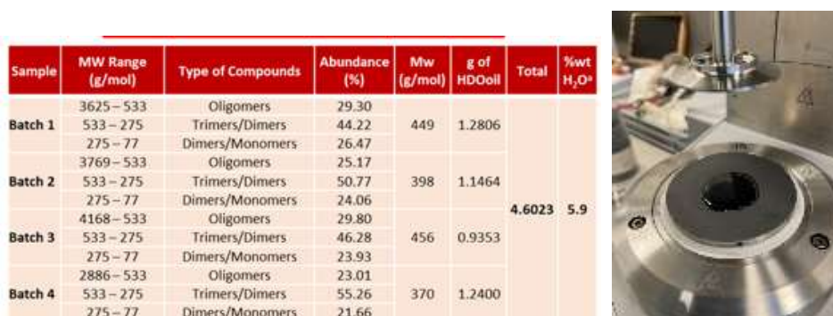
Figure 2. (left) Reproducibility of CLO HDO process with respect the molecular weight distribution of the depolymerized lignin fractions and cumulative production of Bio-HFO for quality control; (right) Bio-HFO produced and analysed for its viscosity.
